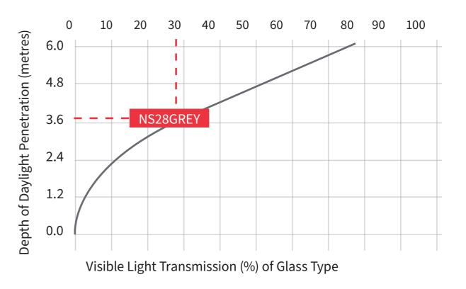
The graph indicates that NS28G applied to clear glass allows an occupant a distance of almost 3.6 metres from the source of light before artificial lighting is required to maintain the 'lighting' level prior to the application of NS28G.
